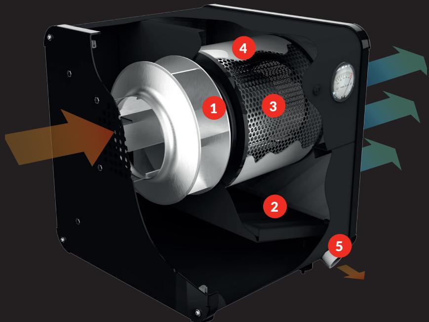
The backward-curved impeller blades (1), specially designed to generate a strong coalescing effect, but above all to prevent any phenomenon of imbalance and consequent vibration throughout the life of the collector, silently direct the airflow inside the mist collector.
